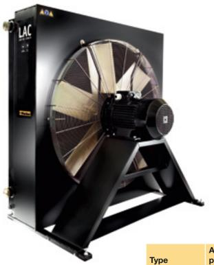
The cooling capacity curves are based on the inlet oil temperature and the ambient air temperature. An oil temperature of 60 °C and an air temperature of 20 °C provide a temperature difference of 40 °C. Multiply by kW/°C for total cooling capacity.
